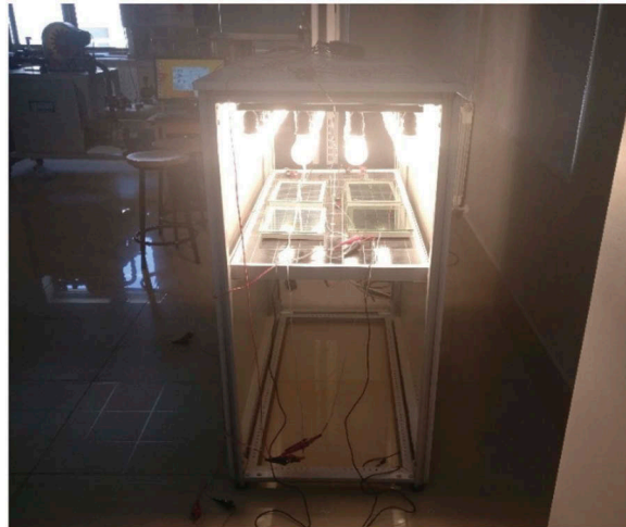
Figure 1. The Photovoltaic Performance Simulator (PVPS) device.
